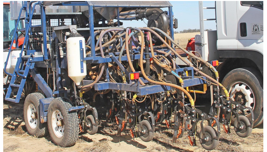
Six row seeder with Ausplow Deep Blade System (DBS) tines
