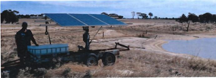
ABOVE: The water pump is powered by 3 solar panels giving a total of 750 watts. They all sit on a trailer which can be moved around the farm as required. Scott said: "We drag pipes and take the solar pump to shift water from where it is to where it's needed."
