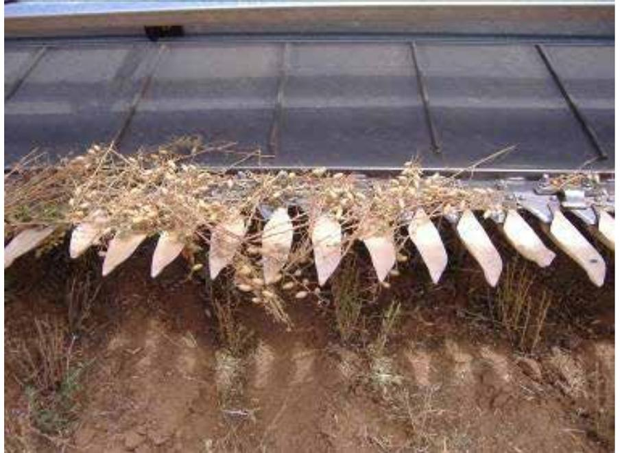
**Photo 3:** Plastic extension fingers fitted to a draper front.
