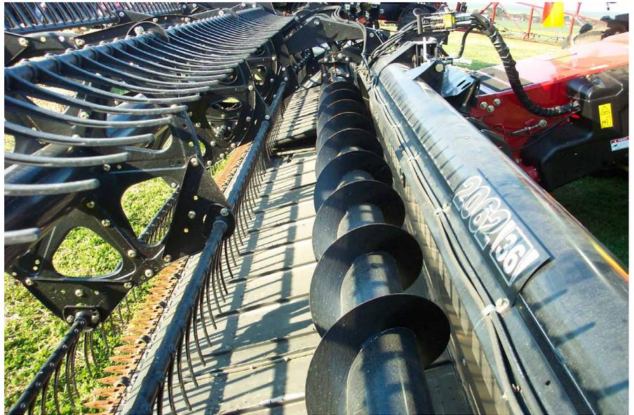
**Photo 1:** Belt-front fitted with cross-auger.
