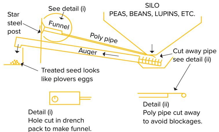
**Figure 2:** Applying inoculum through an auger.
