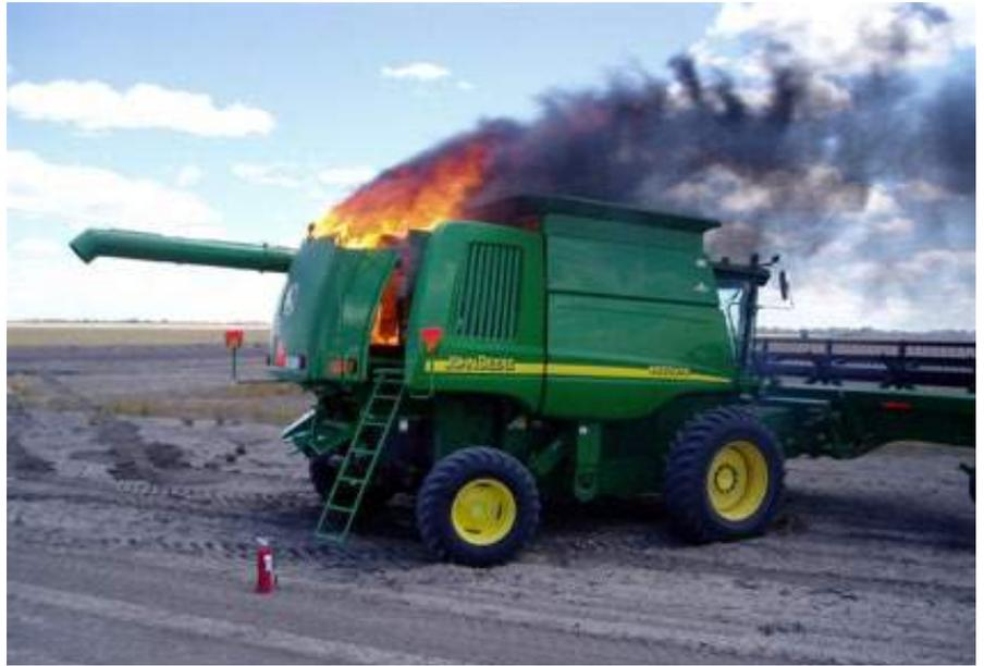
**Photo 17:** A harvester fire in a chickpea crop. This fire took 5 minutes to destroy the harvester.
