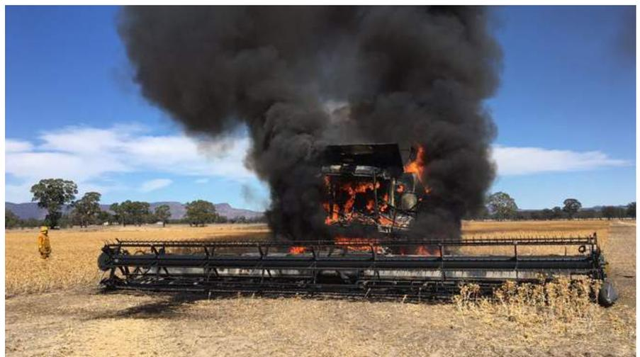
**Photo 16:** A harvester fire in a safflower crop. Like lentil and chickpea, harvesting safflower produces a fine dust meaning the risk of fire is great.
