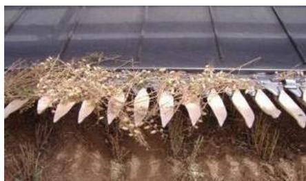
**Photo 6:** Plastic extension fingers fitted to a draper front.
