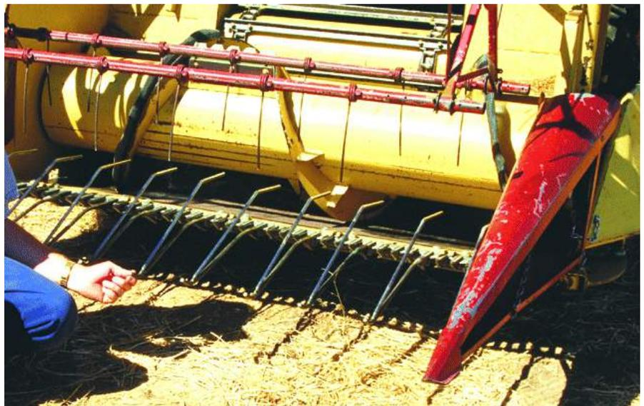
**Photo 5:** Light crop lifters that can be used in lentils.
