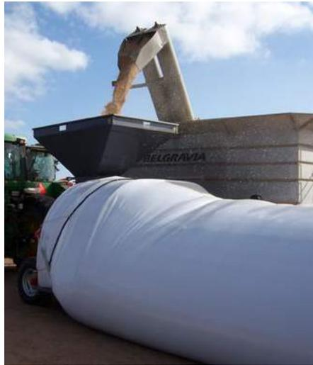
**Photo 6:** Silo bags for lentil storage should be considered as temporary only.
